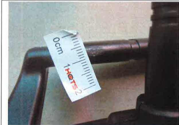
Defect-obvious scratch mark on remote control + poor painting on surface-ma(1)
