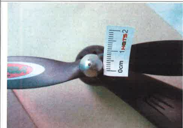
Defect-poor painting on surface-mi(1)
