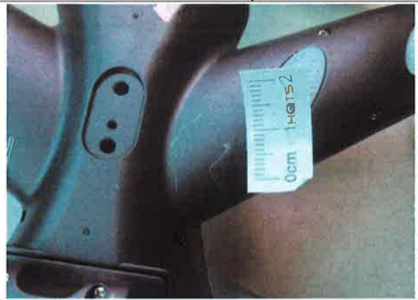
Defect-scratch mark on surface-mi(2)
