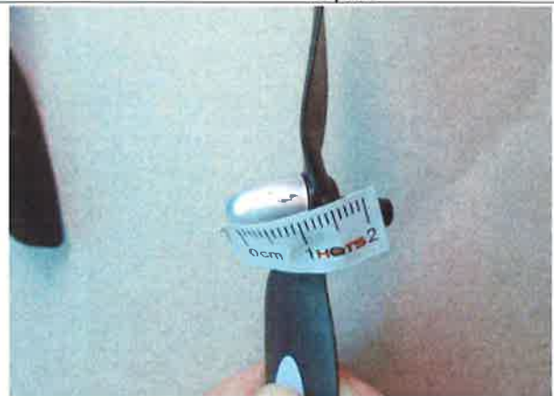
Defect-obvious scratch mark on remote control + poor painting on surface-ma(2)
