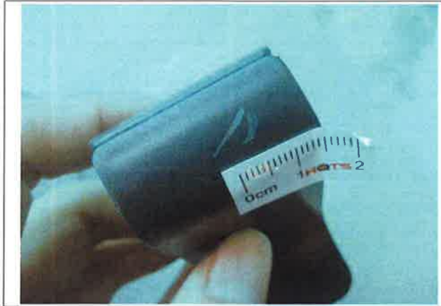
Defect-scratch mark on surface-mi(1)
