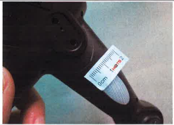
Defect-poor painting on surface + color stain on surface-mi(2)
