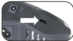
On the left side of the charger is a 3-pin port used as a connection for a temperature sensor (not included). If the screen displays temperature, you can use the optional temperature probe to connect to the surface of the battery. **The USB function is not available for this charger.**
